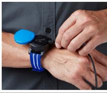
5. Insert the transducer inside the transducer holder so that the serial number is visible.
